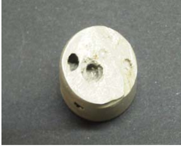
Figure 1 Photo showing the cavities of a composite with 80 % (w/w) of silver.
